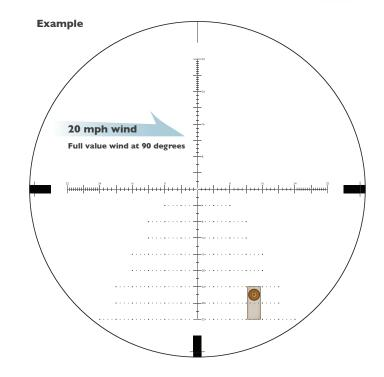
14 MOA reticle windage correction for 20 mph wind at 800 yards using the 26 MOA reticle drop line.
