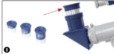
8 Finally, select one of the three eyepieces and fix it to the zenith mirror (or on the eyepiece extender).
